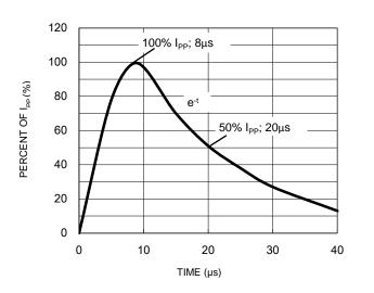
Fig.7 ESD pulse waveform per IEC61000-4-2
